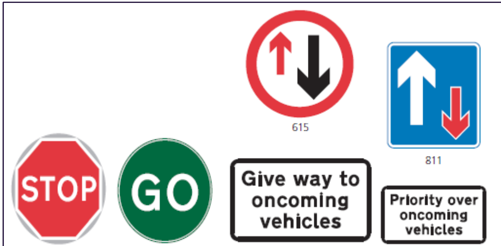
Figure 1.7: Manually operated stop/go signs and priority signs.
